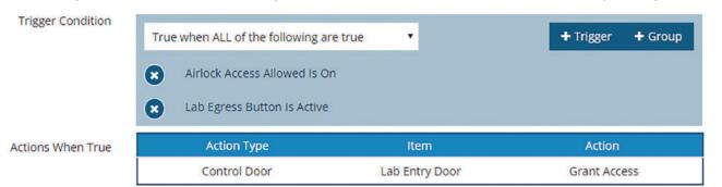
This action will grant access to the *Lab Entry Door* (unlock for the default unlock time) when the *Lab Egress Button* is pressed, but only if the *Airlock Access Allowed* custom output is on. A similar automated action can be made for the other egress button to leave the airlock.
