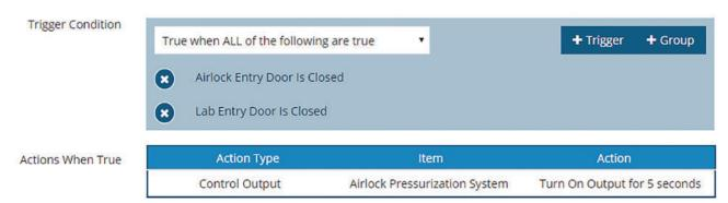
As the triggers are edge based, the output will only turn on when both doors are closed, after one was opened.
