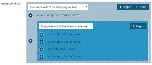
If the emergency override input is active, then the *Airlock Access Allowed* custom output will always be on, ignoring the states of the doors. This lets all of the other logic using this custom output to remain unchanged.
