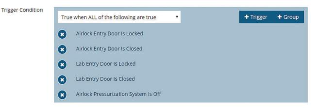
The pressurization system can then be controlled by another automated action where when both doors are closed, the system is run for 5 seconds.
